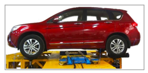
Couple our 94 Series actuators and high precision three stage servo valves with Real Time Active Control (RTAC) and you have the perfect ingredients for a reliable, easy to use and accurate Four Post Road Simulator. Push button reproduction of spindle acceleration means that novice operators can recreate road profiles easily, without long-winded training or specialized personnel.
