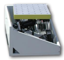
We are even able to control **multiple tables as a single plane.** The user can freely switch between actuator commands and cartesian commands, depending on their preference for the given task.
