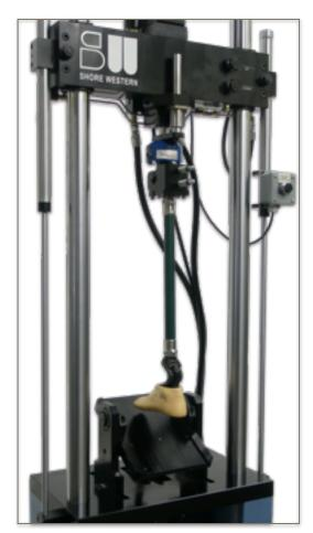
Our Real Time Active Control (RTAC) algorithm is adept at **reproducing highly non-linear forces.** For example, the force in a walking foot is controlled and adjusted in real time via the angle of the lower platen and the vertical actuator position. A capability not shared by our competitors.
